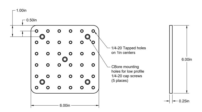
True  $\frac{1}{2}$  Inch border so breadboards can be stacked without losing hole spacing.
